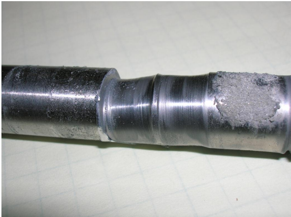
Figure 4.5 Close up for Sand in Shaft Grind Wear
