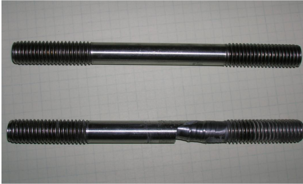
Figure 4.4 Comparison between Shaft Grind Wear, new and old
