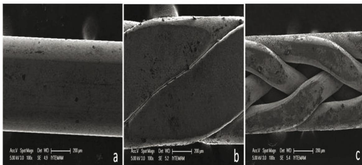
**Figure 2.** SEM micrographs of  $\text{TiO}_2$  anatase film on orthodontic arch wire surfaces: a)  $0.016 \times 0.022$  inch stainless steel wire, b)  $0.016 \times 0.022$  inch D-rect wire, c) multistranded hammered retainer wire.
