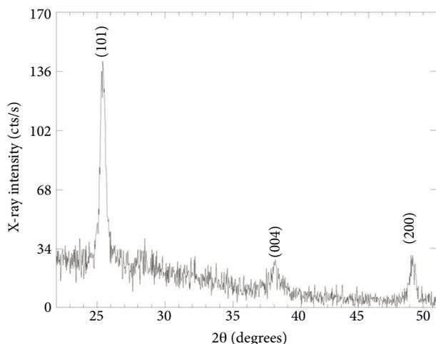
**Figure 1.** GIXRD spectra of  $\text{TiO}_2$ -coated glass substrate after heat treatment at  $500\text{ }^\circ\text{C}$ .
