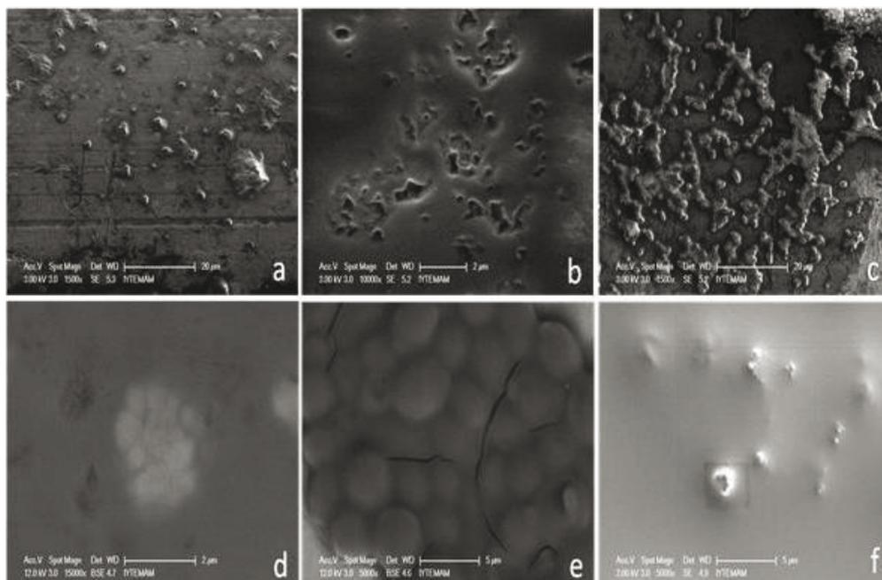
**Figure 3.** Photocatalytic effect of most potent anatase-film-coated orthodontic wires on *S. mutans*, *E. faecalis*, and *C. albicans* in SEM observations: *S. mutans* cells on TiO<sub>2</sub> anatase-film-coated stainless steel wire before (a) and after (b) UVA illumination. *E. faecalis* on multistranded hammered retainer wire before (c) and after (d) UVA illumination. *C. albicans* on multistranded hammered retainer wire before (e) and after (f) UVA illumination.
