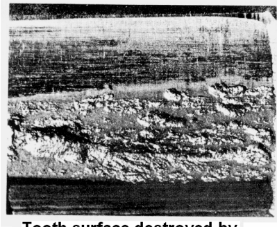
Tooth surface destroyed by extensive pitting.
