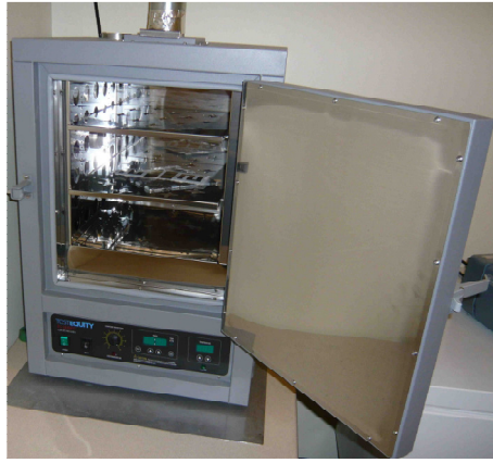
Figure 7. Test Equity FS series industrial oven for performing curing of the prototype antenna
