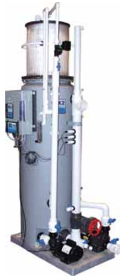
In this foam fractionation unit, one pump moves water through the unit for the treatment process, while the second pump drives a venturi that injects air into the base to create bubbles that rise and create foam at the top.
