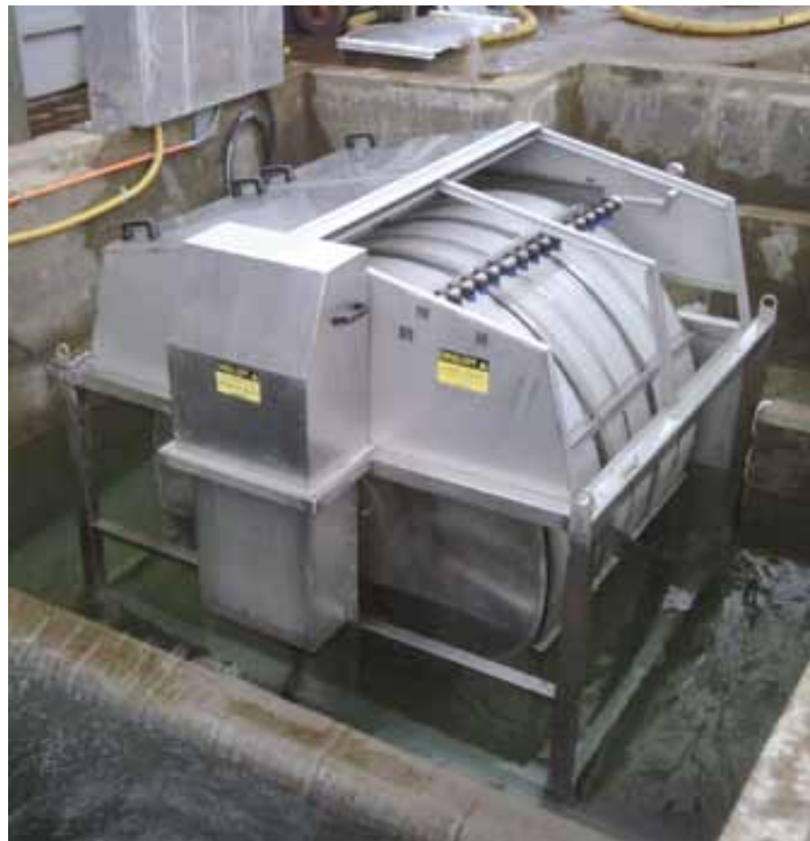
Commercial drum-screen filters remove suspended solids from RAS production systems.
