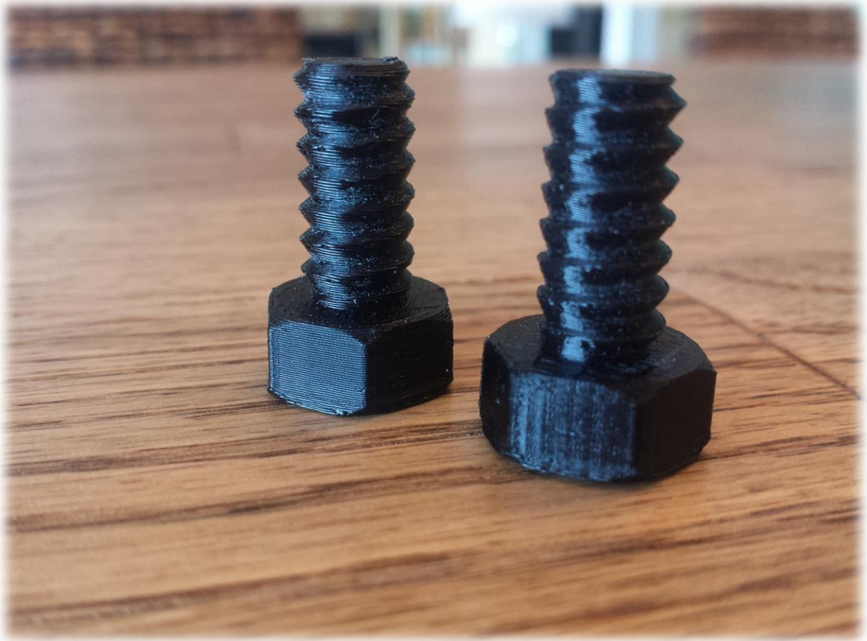
Left: .2mm Layer Height. Right: .1mm Layer Height
