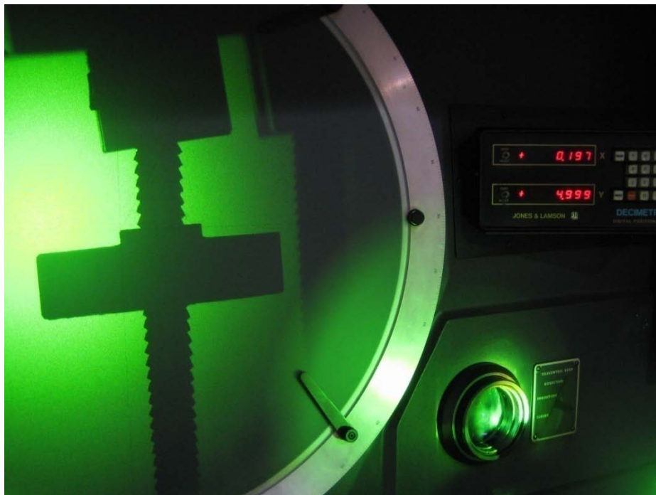
Figure 35: The shadow projected on the screen after the device has made a movement. The digital readout is located on the right.
