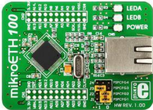
Figure 6: Mikroelektronika's 100Mbps mikroETH100 Ethernet Board, using Microchip's ENC624J600 10/100 Base-T Ethernet controller.
