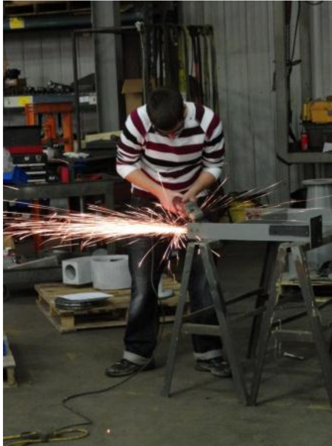
Figure 11: Frame Preparation for Painting
