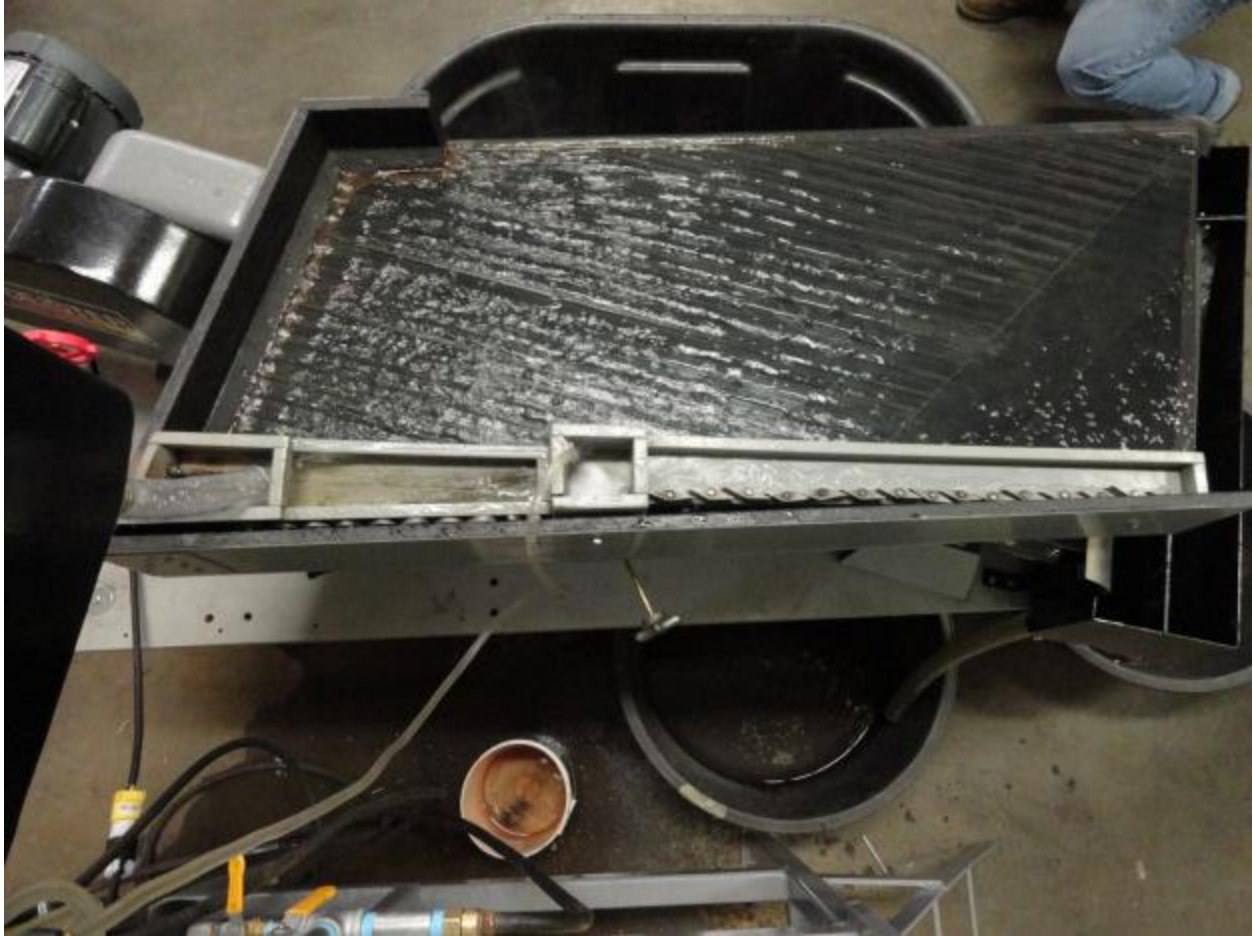
Figure 61: Water Flowing from Mixing Hopper, to Feedbox, across the Table, and Into the Collection Bins
