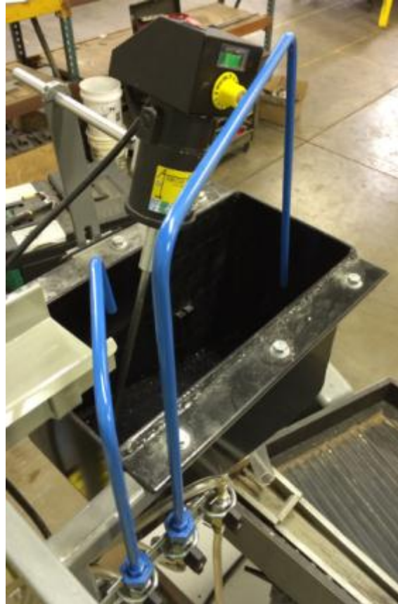
Figure 44: Top View of Hopper with Placement of Pipes and Mixer
