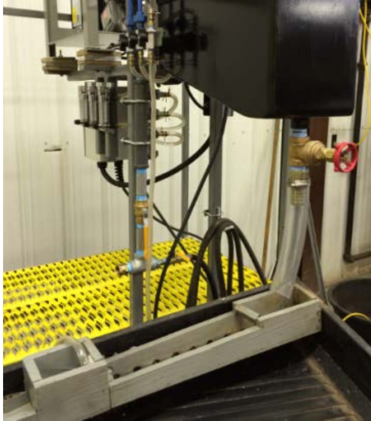
Figure 47: Wash Water and Slurry Flow Entering the Un-modified Table
