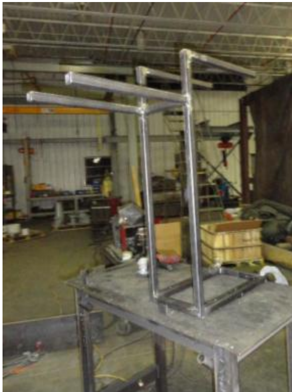
Figure 15: Welded Frame Ready for Paint
