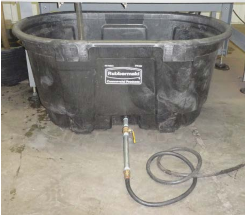
Figure 48: Tailing Collection Bin with Drain Hose
