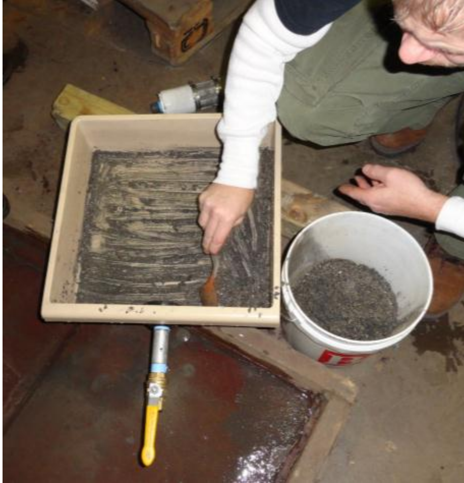
Figure 63: Tailing Material that was Captured by the Filter
