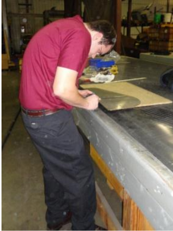
Figure 17: Marking Mounting Plates
