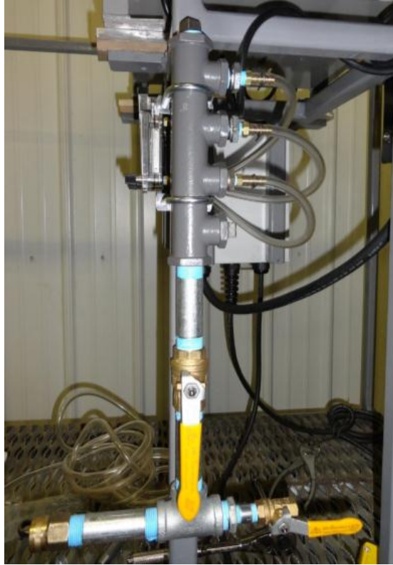
Figure 39: Water Supply System – Main Distribution Piping
