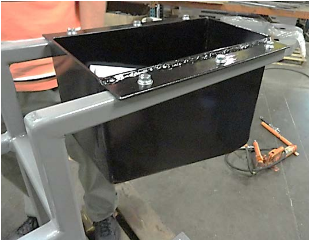
Figure 32: Mixing Hopper Secured Frame with Six 5/16"-18 Bolts and Locking Washers
