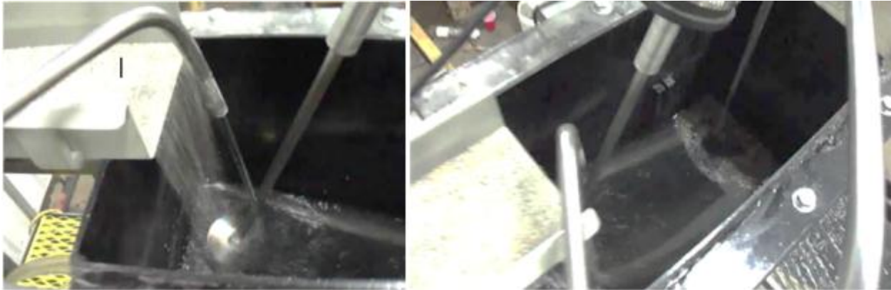
Figure 37: To Accommodate a Rocky Sample, Tilting the Mixer into the Feed and Removing the Hopper Baffle Resulted in Optimal Performance
