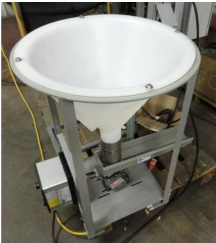
Figure 28: The Vibratory Feeder as Received
