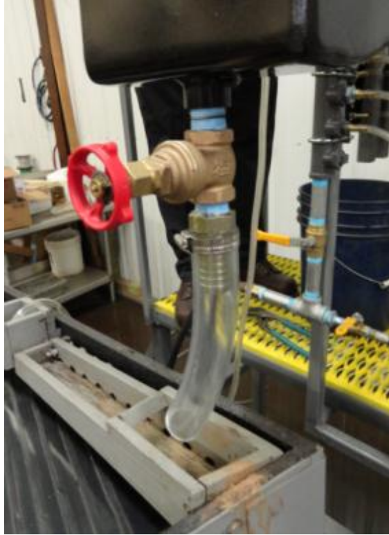
Figure 45: Drain Hose from Hopper to Feedbox
