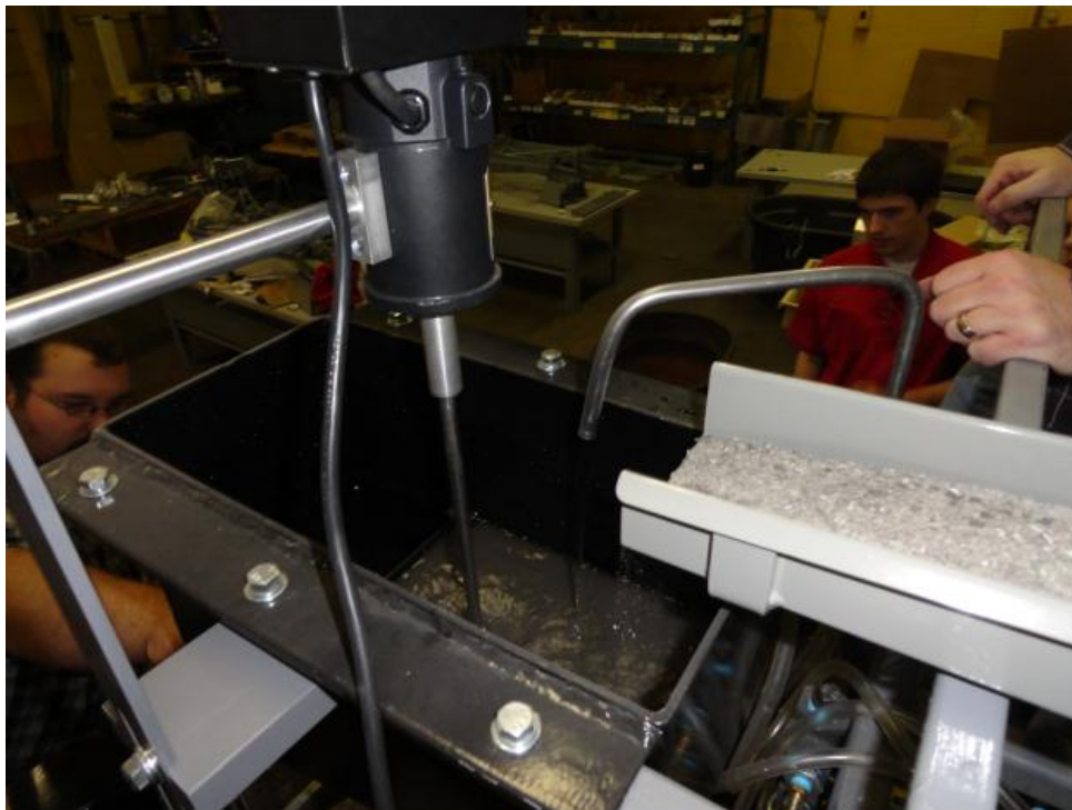
Figure 65: Material from Feed System Entering Mixing Hopper
