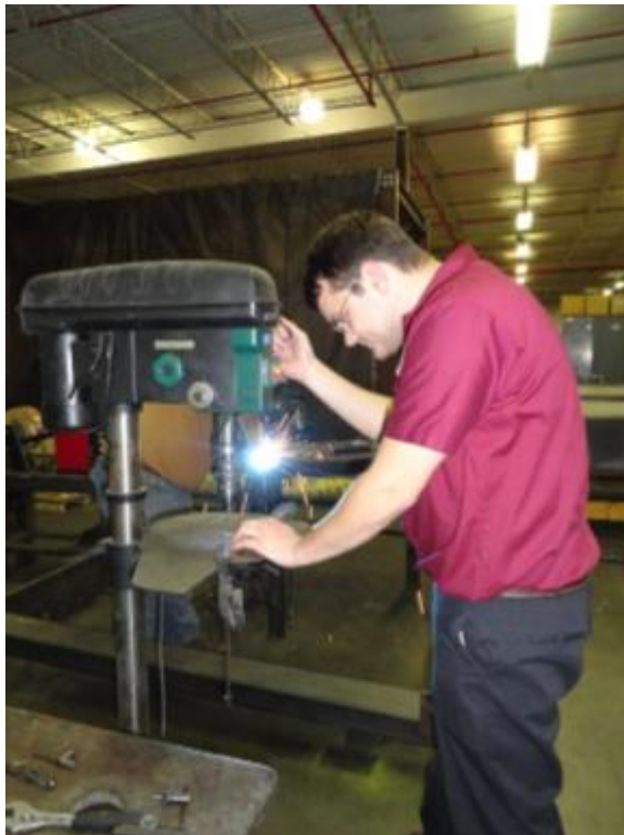
Figure 18: Drilling Mounting Holes
