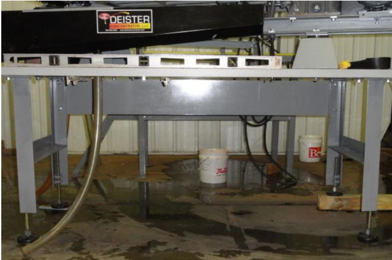
Figure 66: Table Shown on Simulated Uneven Ground
