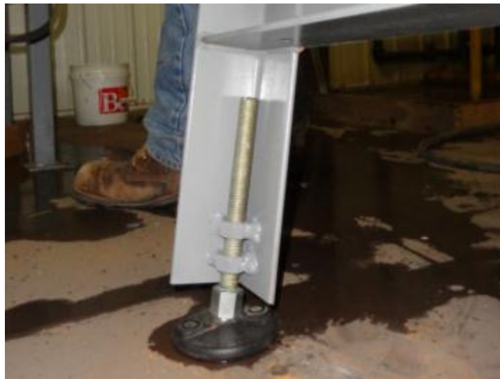
Figure 12: Finished Adjustable Legs
