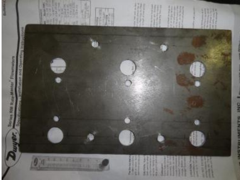
Figure 19: Mounting Plate Ready for Paint
