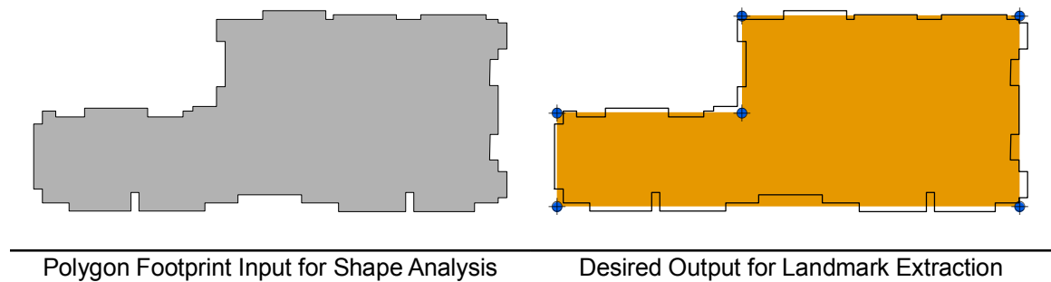
Figure 3.14 -- Desired landmark outputs that mimic human judgment
