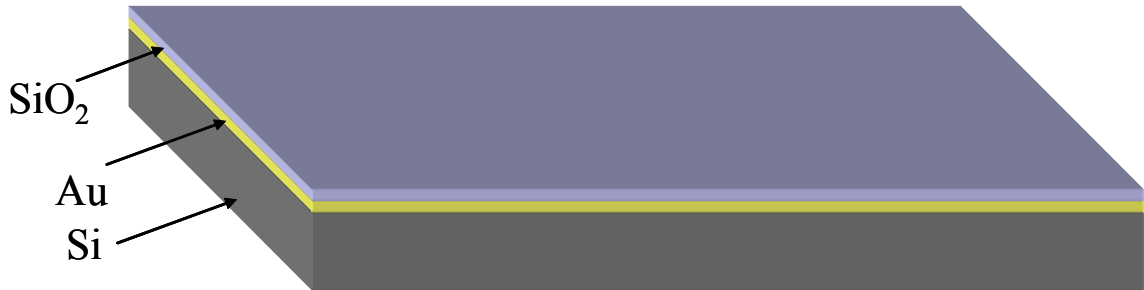
Figure 4.4 \text{SiO}_2 insulation layer deposited using PECVD.
