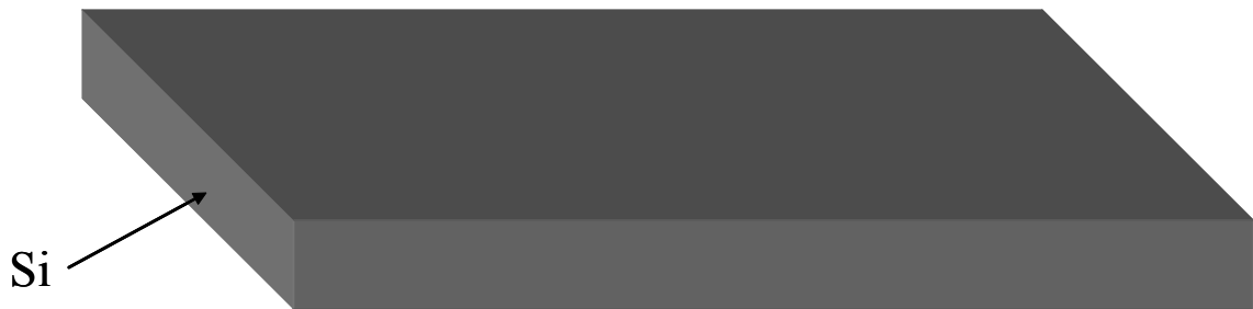
Figure 4.21 Step1—Double-sided polished Si wafer.
