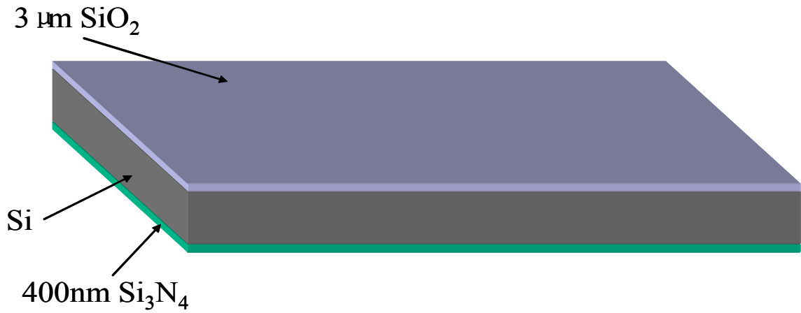
Figure 4.23 Step3—PECVD nitride is deposited on the back-side.
