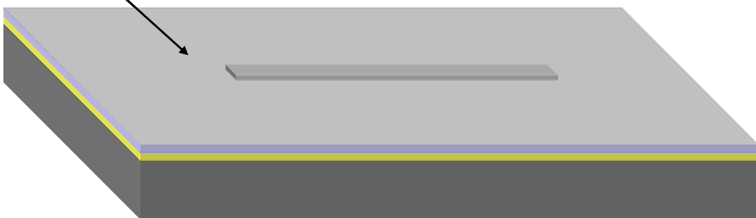
Figure 4.11 Sputtering of aluminum to conformally coat the belt and wafer.
