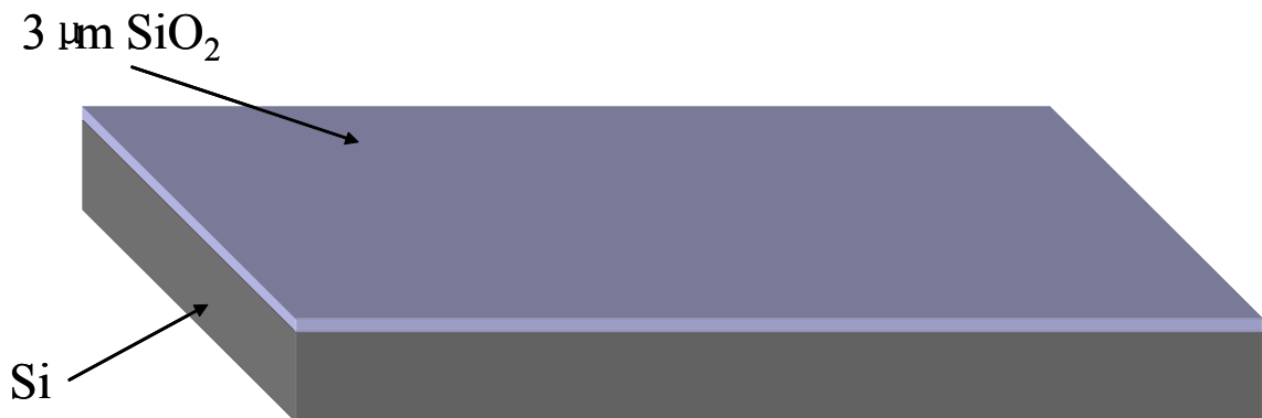
Figure 4.21 Step1—Double-sided polished Si wafer.
