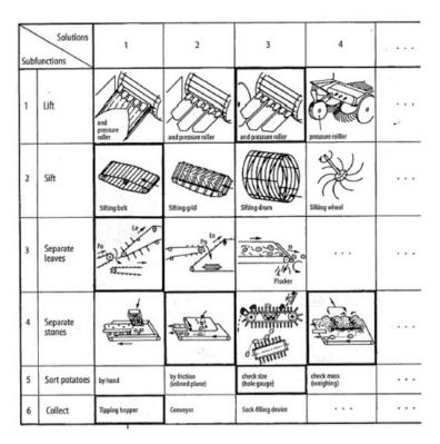
Figure 2.3 Morphological matrix for potato harvesting machine [5]
