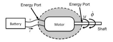
Figure 2.8 Electric Motor Example
