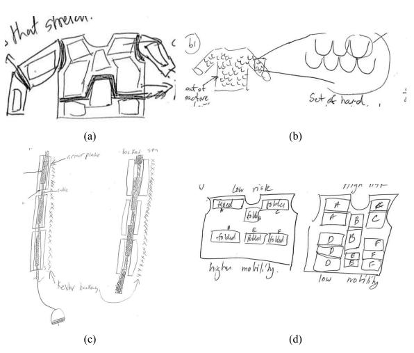
Figure 7.5 Sample design solutions from Study 2 (a) Segmented armor (b) armor scales (c) pull-string activated variable-stiffness armor (d) foldable armor plates
