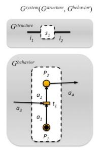
Figure 3.11 Petri Net System Model
