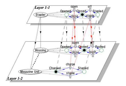
Figure 2.11 Hierarchical Petri net representation for a stapler design [60]
