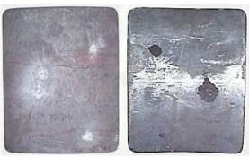
Figure 7.6 Steel armor plates for hard body armor
