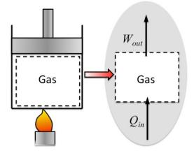
Figure 3.5 Piston-Cylinder Assembly
