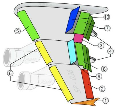
Figure 8.8 High-lift features – (1) Wingtip, (2) Low Speed Aileron, (3) High Speed Aileron, (4) Flap track fairing, (5) Krüger flaps, (6) Slats, (7) Three slotted inner flaps, (8) Three slotted outer flaps, (9) Spoilers, and (10) Spoilers Air-brakes [172]
