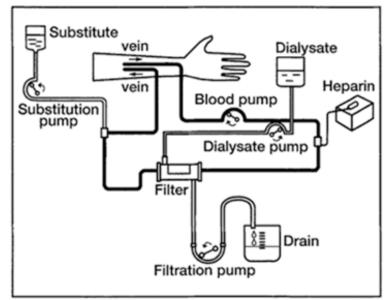
Figure 8.13 Hemodiafiltration circuit [179]
