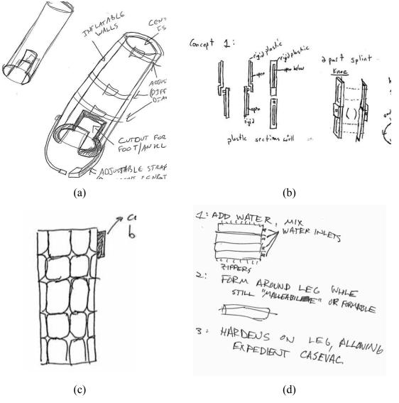
Figure 7.3 Sample of design ideas from Study 1 (a) Inflatable (b) multiple-part snap (c) electrorheological fluid chambers with power source (d) chemically-rigidizable
