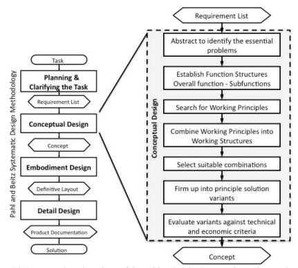
Figure 6.2 Conceptual Design phase of the Pahl and Beitz Systematic Design Methodology
