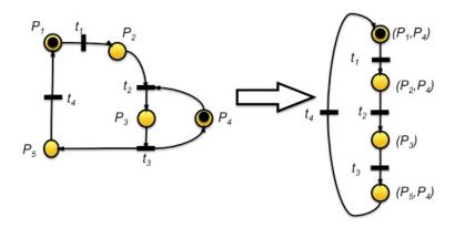
Figure 4.5 Reachability graph example: (a) Petri net model and (b) Reachability graph
