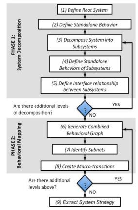
Figure 4.8 Flowchart for Method for Reverse Engineering Biological Systems
