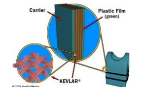
Figure 7.7 Kevlar® based Soft Body Armor (HowStuffWorks)
