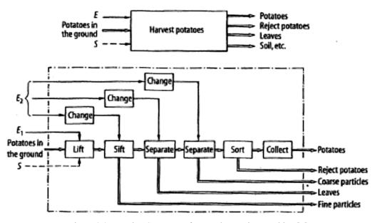
Figure 2.2 Function Structure of potato harvesting machine [5]
