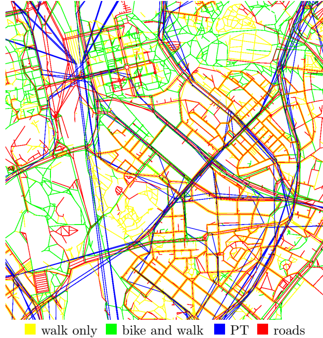
Figure 5.2: Visualisation of a 2.4 km by 2.4 km fragment of the Helsinki GTD graph. Edge colours denote the modes of transport permitted at each edge, cf. legend. All other combinations of modes (e.g., car and taxi, bike only) are marked red. There are approximately 9 500 nodes and 27 700 edges in the visualisation.
