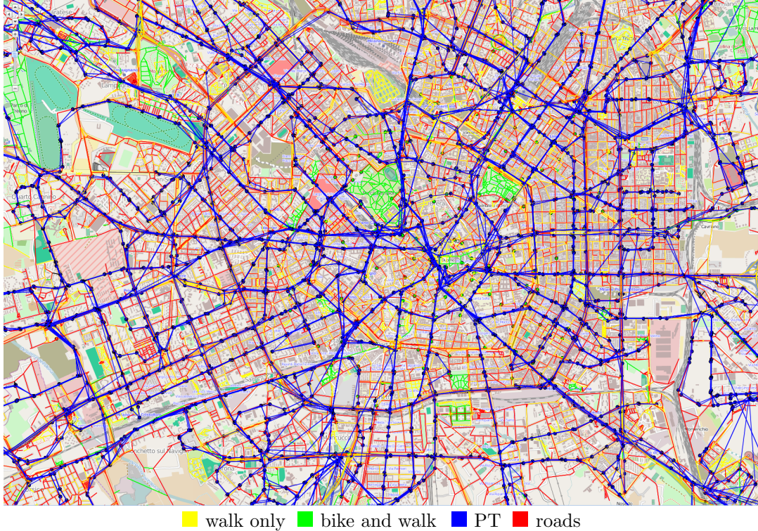
Figure 5.6: GTD graph of Milan (221 707 nodes and 601 695 edges).
