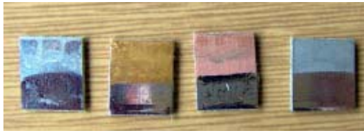
Fig. 5. Photo of the used samples (with different surface finishes) after measurement.
