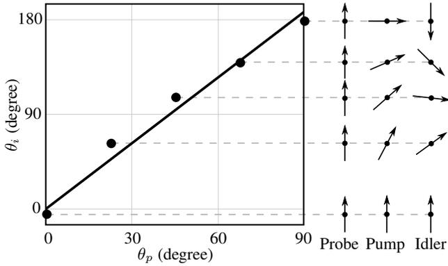
FIG. 9. Linear polarisation angle  $\theta_i$  of the idler as a function of the linear polarisation angle of the pump  $\theta_p$ . The linear polarisation of the probe is kept vertical while the pump angle is rotated from 0 degree (parallel to the probe) to 90 degrees (perpendicular). The dots are the experimental data points. The solid line is a fit with  $\theta_i = 2\theta_p - \theta_s$ .
