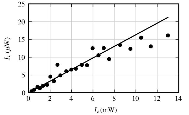
FIG. 6. Idler power  $I_i$  plotted against the probe power  $I_s$ . The dots are experimental data points, the solid curve is a linear fit to the low power data. See the text for the value of the fixed parameters.
