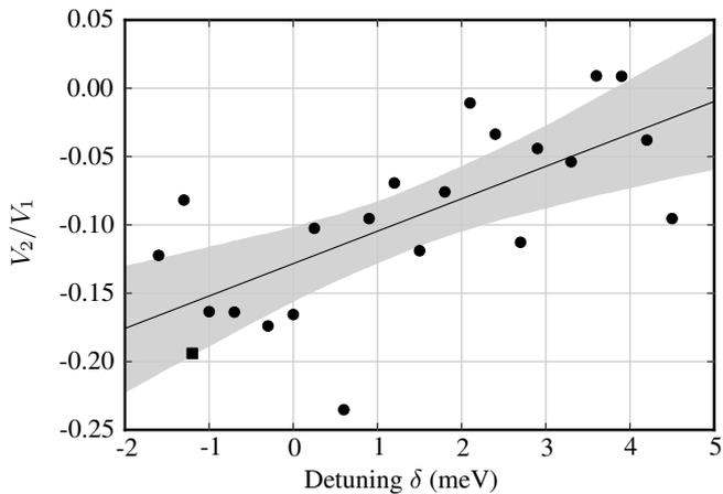
FIG. 12. Ratio  $V_2/V_1$  of the polarisation-dependent scattering strengths measured over a range of laser-exciton detunings  $\delta = E_p - E_X$ . The square data point corresponds to the measurements presented in Fig. 10. The solid line is a linear regression. The shaded area is a 95% confidence region for this linear regression, bounded by the 2.5% and 97.5% quantiles.
