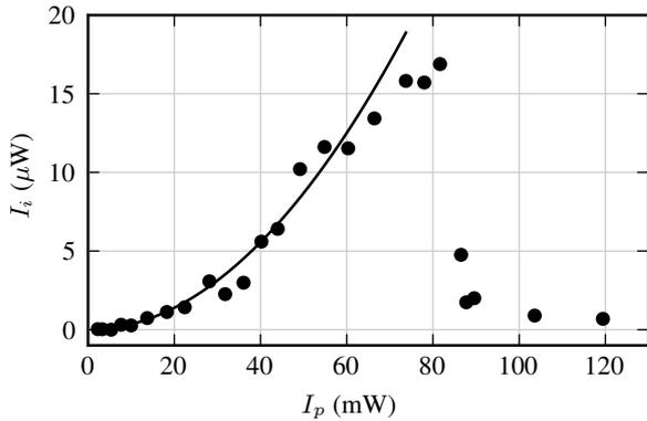
FIG. 7. Idler intensity  $I_i$  plotted against the pump power  $I_p$ . The dots are experimental data points, the solid curve is a square-law fit to the low-power data.
