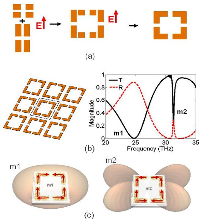
**Figure 2.** (a) The transformation from an 8-gap-multi-gap split ring resonator (MSRR) and its corresponding equivalent resonators under a linearly polarized incident wave to the 4-gap MSRR with four-fold symmetry. (b) Schematic view of the metamaterial composed of an array of metallic MSRRs (left) and Transmission and reflection spectra of the MSRR (right). (c) Cartographies of the surface current and the radiation patterns of the MSRR at the two first resonances.
