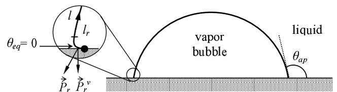
FIG. 2: Apparent ( $\theta_{ap}$ ) and actual ( $\theta_{eq}$ ) contact angles. The solid circle indicates the contact line, the zero point for the curvilinear coordinate  $l$  measured along the bubble contour. The arrows show the directions of the vapor recoil force in the vicinity of the contact line and its vertical component that creates an additional adhesion of the bubble to the heater.
