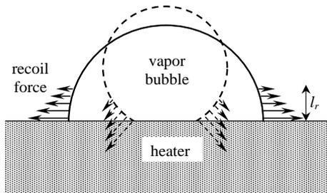
FIG. 1: Sketch illustrating the vapor recoil effect. The amplitude and direction of the vapor recoil force are shown by arrows. The thickness  $l_r$  of the belt on the bubble surface, in which the vapor recoil force is important, is exaggerated with respect to the bubble size.
