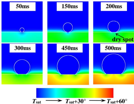
FIG. 3: Vapor bubble spreading under the influence of vapor recoil simulated for water at 10 MPa. The color indicates the local temperature with respect to the saturation temperature  $T_{sat} = 311^\circ\text{C}$ ;  $q = 0.1 \text{ MW/m}^2$ .
