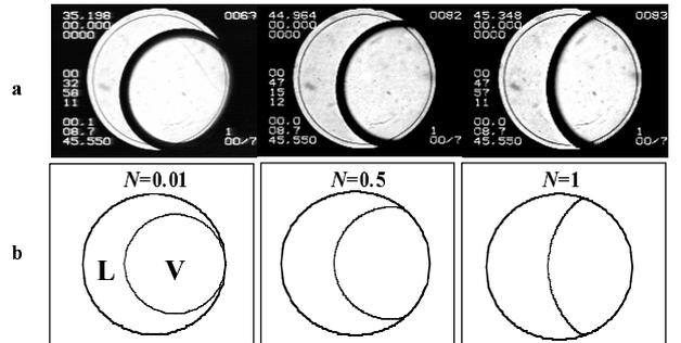
FIG. 4: Snapshots of the vapor bubble (V) growing in near critical liquid (L), both experimental (a) and calculated (b) for the given values of the vapor recoil strength  $N$ . The zero value of the actual contact angle is imposed while the apparent contact angle attains a large value.
