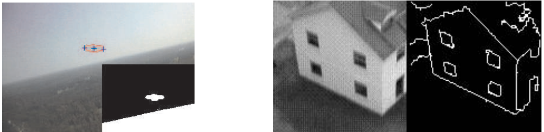
Figure 2: Examples of Image Processing: (Left) Detecting an airplane flying ahead, (Right) Detecting edges of a ground obstacle
