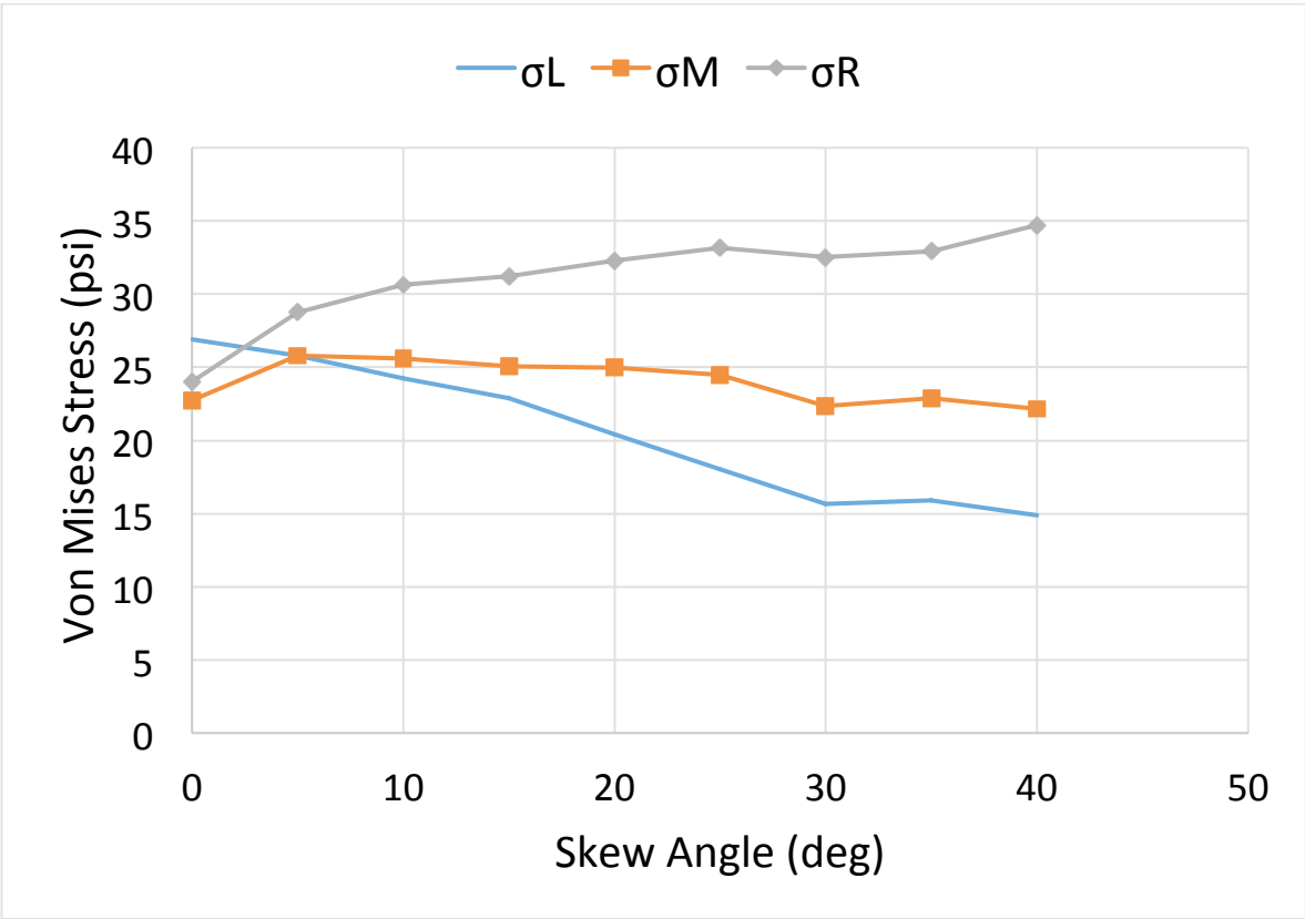
Figure 6-36: Von Mises stress values within the RBS with radius cut parallel to the column flange for skewed configurations at 50% yield.
