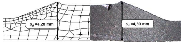
Figure 4 Simulated and experimental geometry of the forming zone
