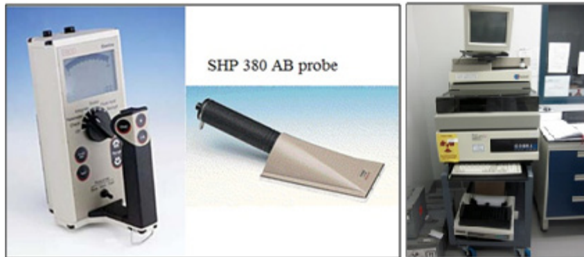
Figure 30 Eberline-E600 (left) and Cobra Packard II multisampling (right) detectors used on the experiments.
