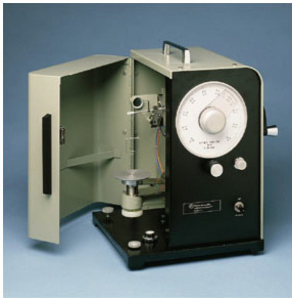
Figure 16 Fisher Semiautomatic Model 21 Tensiomat used to measured surface tension
