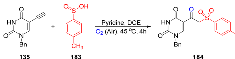
Scheme 51. Synthesis of 5-( \beta -keto)sulfonyluracil via aerobic difunctionalization of 5-ethynyluracil 135
