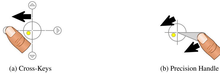
Figure II.1: Examples of the Cross-Keys (a) and Precision Handle (b) techniques for indirect selection where the task is to select the circular target. (Albinsson and Zhai, 2003a).
