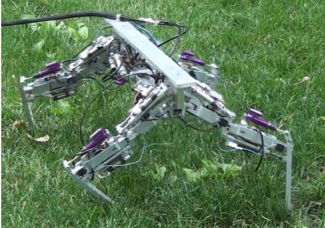
Fig. 49. Final design and construction of the quadrupedal pneumatic robot traversing a grass substrate.
