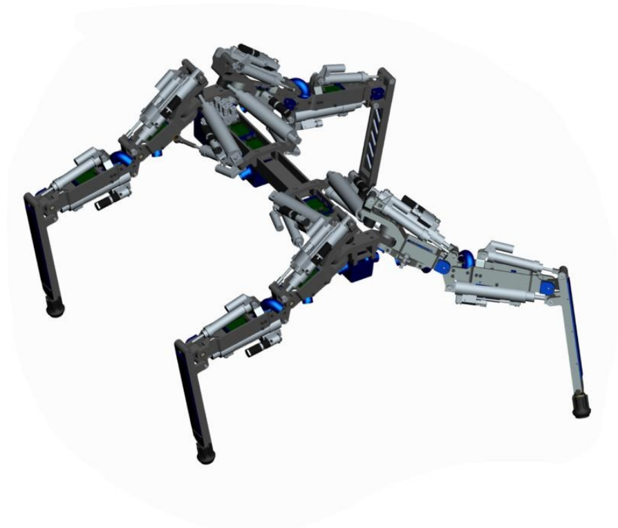
Fig. 41. Final, as-built design of quadrupedal robot. Shown without fuel tank, batteries, or on-board high level computation.
