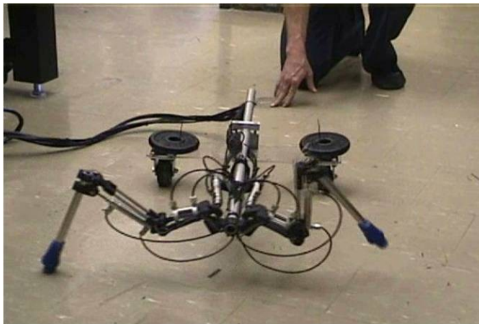
Fig. 18. Initial, position controlled two-legged prototype
