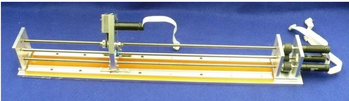
Figure 6.5: The robotic actuation unit, showing the carriage, which can move independently when actuated by lead screws coupled to the motors pictured to the far right in the image. Only a single motor is used for this purpose. Other two enable the addition of additional carriages for multi-lumen needles. The needle is attached to the carriage, which carries motor and belt drive assembly to rotate the tube axially.
