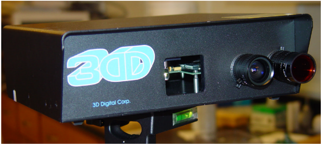
Figure II.1: Laser scanner used to acquire textured point clouds.
