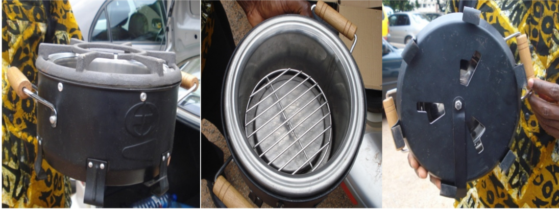
Figure 4-3: Envirofit charcoal cookstove showing the external view, interior and the base Source: Author's field survey, July 2012
