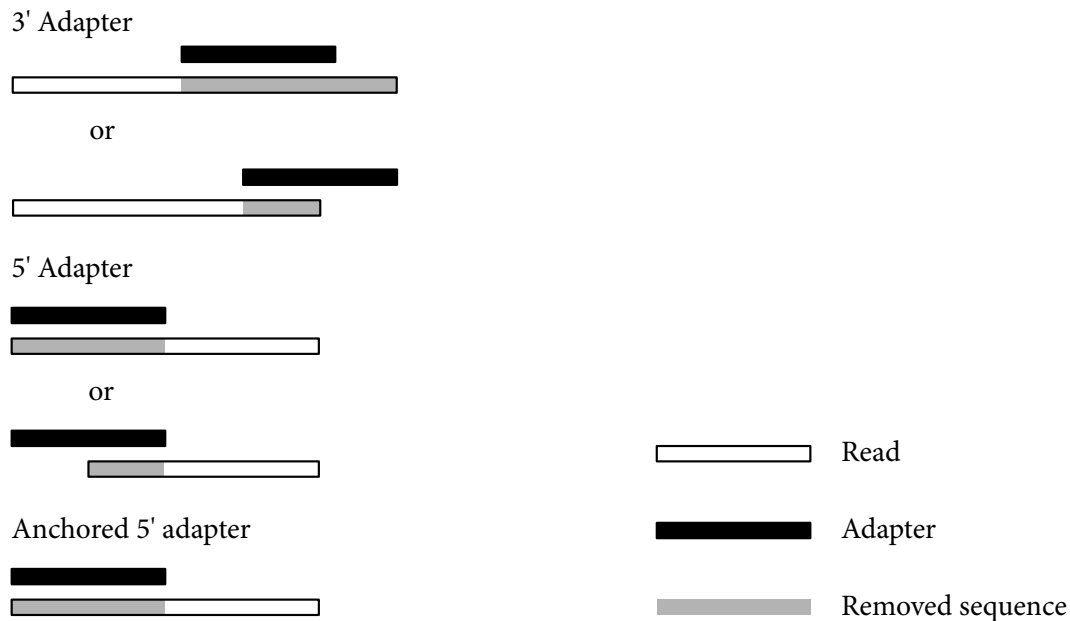
Figure 2.1 Types of adapters, how they appear within reads, and which part of the read needs to be removed if the adapter is found. A mixed adapter may appear in any of the shown configurations.
