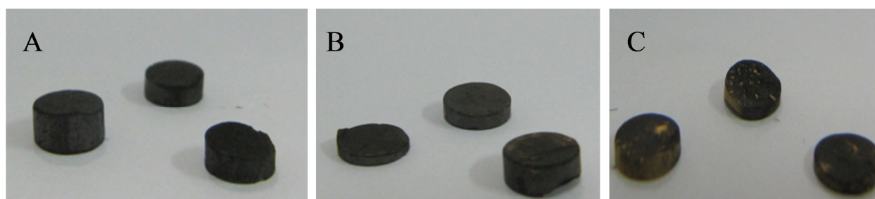
Figure II.4.4. Morphologie des disques de carbones poreux C-HIPE (60Carb) (A), 5-Au@C-HIPE (60Carb) (B), 15-Au@C-HIPE (60Carb) (C).
