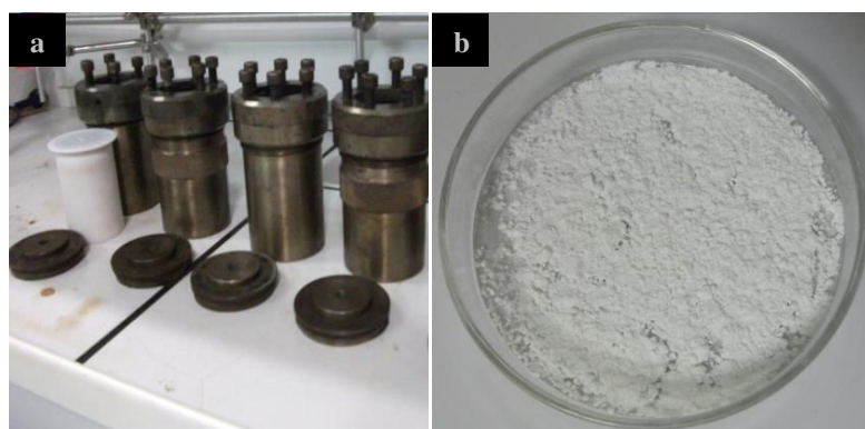
Figure 4.3 - (a) Teflon lined steel autoclave of 125 mL for ZIF-8 synthesis; (b) Sample of ZIF-8 as-synthesized.
