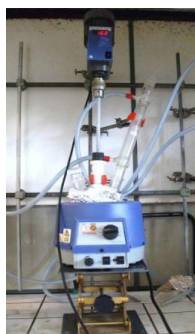
Figure 1.12 - Experimental set-up for the bottom flask synthesis.
