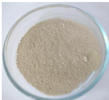
Figure 5.5 - Final product of the sample MIL-53(Fe)–(CF 3 ) 2 after calcination.
