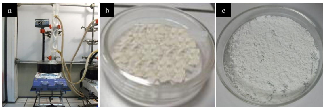
Figure 3.6 - (a) Experimental set-up used for UiO-66(Zr)-NO 2 synthesis; (b) Sample of UiO-66(Zr)-NO 2 as-synthesized (c) Final product after activation.
