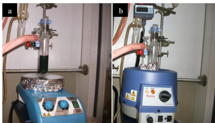
Figure 6.8 - Experimental set-up for (a) pure ethylamine grafted at room temperature and (b) aqueous ethylamine grafted at around 373 K.
