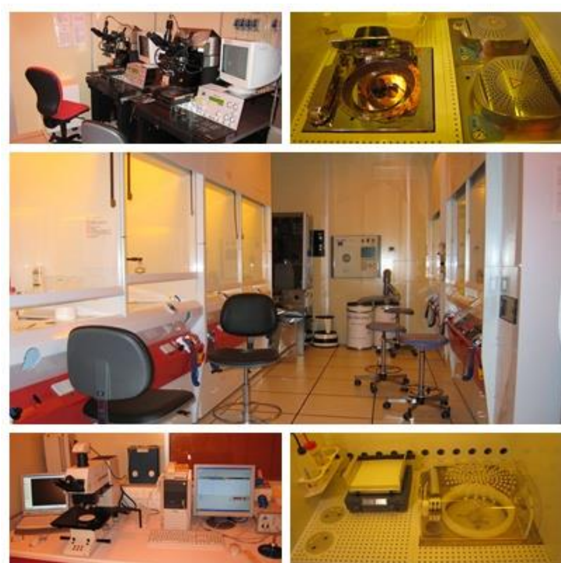
FIG. 4.5. Photolithography in the clean room of IEMN.
