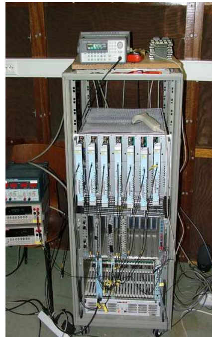
Figure 5.7: Photograph of the test board card (right) and the calibration system (left) for the VFE cards developed and used at IPN Lyon.
