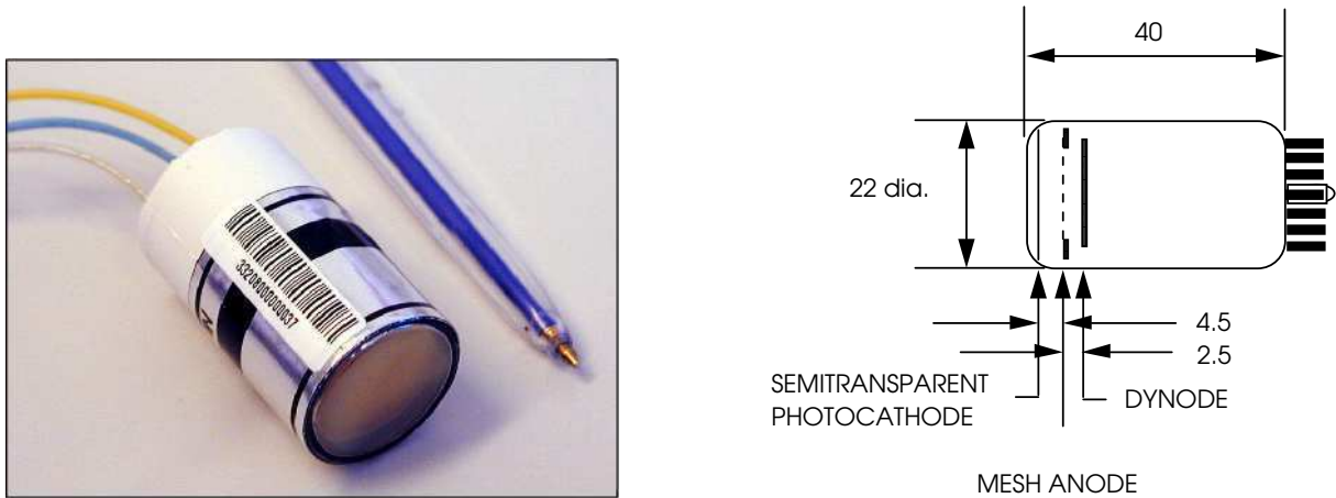
Figure 2.8: Left: A photograph of the CMS vacuum phototriodes (VPT). Right: Schematic view of the VPT.
