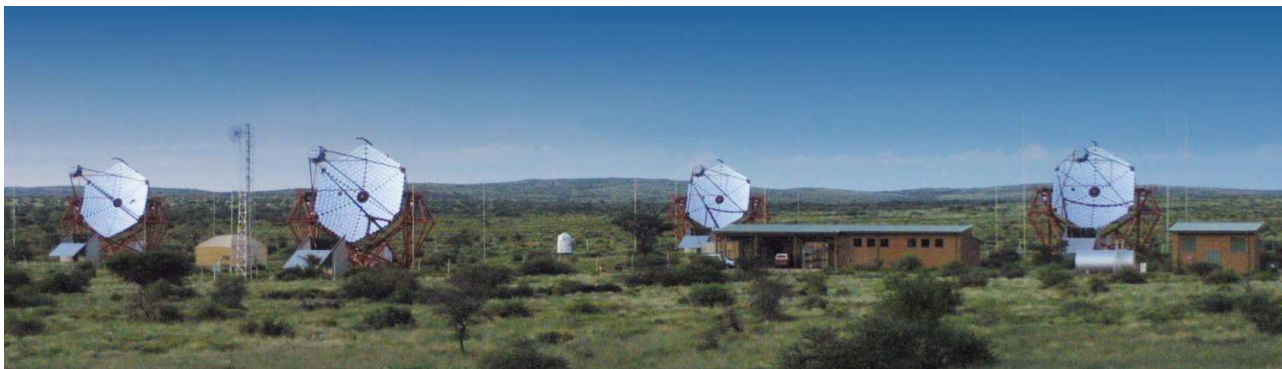
Figure 1.12: The HESS telescope array, located in Namibia, is an array of four imaging atmospheric Čerenkov telescopes separated by a 120 m baseline which allows an optimal triangulation of the . Each of these telescopes is equipped with a tessellated spherical mirror of 107 m 2 area and a camera comprised of 960 photomultiplier tubes, covering a 5° fov. The system works in a coincidence mode [Funk et al., 2004], requiring at least two of the four telescopes to trigger the detection of a cascade. This stereoscopic approach results in a high angular resolution of 5' per event, and an energy resolution of 6% on average.
