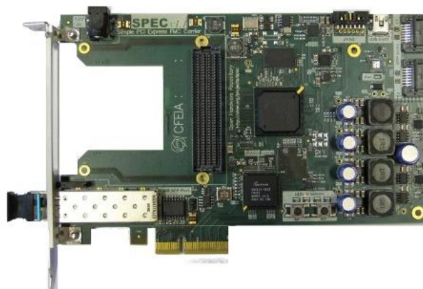
Figure 6.59: The Simple FMC carrier (SPEC) card with the PCI press interconnection and the Xilinx FPGA [81].
