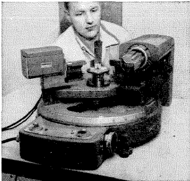
Engineer measures residual stress in a compressor blade non-destructively, using X-ray diffraction. Stress analysis plays important part in developing advanced aircraft engine designs.
