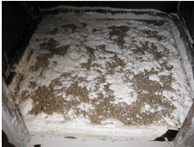
Figure (5.18) Interface of the sand sub-base after test
