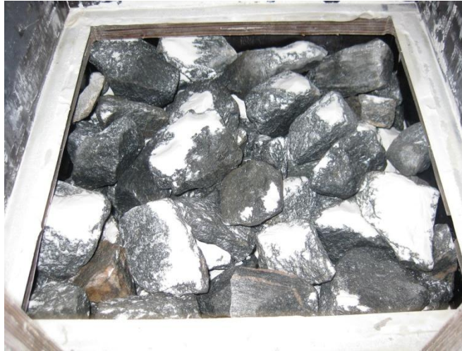
Figure (5.19) Interface of the stone sub-base after test
