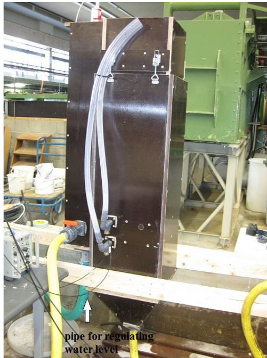
Figure (5.15) Water level regulation by the pipe
