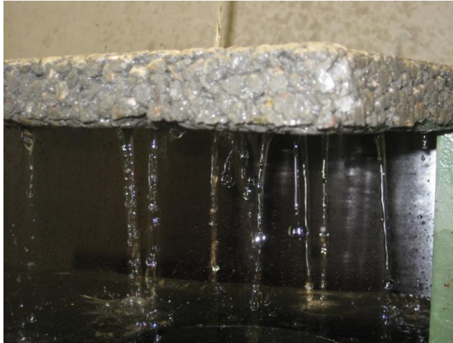
Figure (5.10) Flow through the tile
