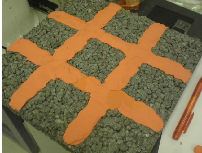
Figure (5.9), filling the gaps of the tile with clay to measure the porosity
