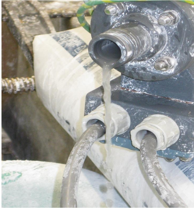
Figure (5.20) Small flow in test with M6.1, sand sub-base
