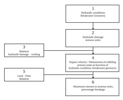
Figure 2.1: Calculation Procedure (CUR, 1990a)
