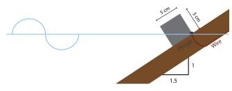
Figure 4.1: Illustration experimental setup - side view
