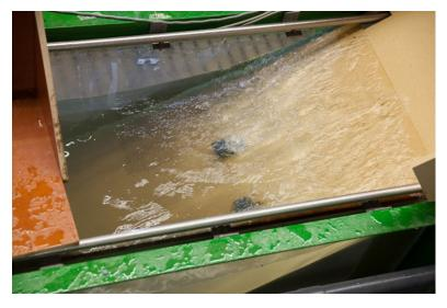
Figure C.3: Wave run-up for exposed cubes. No movement
