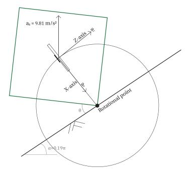
Figure 8.1: Alignment accelerometer axes parallel to the tangential and normal acceleration
