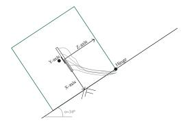
Figure 4.9: Orientation accelerometer inside cube
