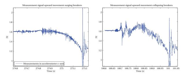
Figure 6.9: Comparison of the signals of upward movement under surging and collapsing breaker conditions
