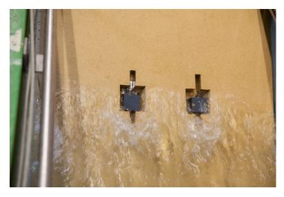
Figure C.5: Wave run-up for the embedded cubes
