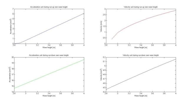
Figure I.6: Resulting accelerations and velocities varying over wave height of prototype Hexapod with orientation 1
