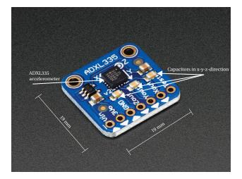
Figure 4.8: Accelerometer ADXL335 (Adafruit, n.d.)
