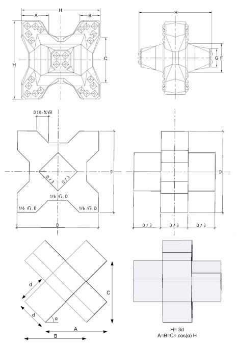
Figure I.1: Front and side view of the Accropode 2 (top) (CLI, 2011), Xbloc (middle) (Zwanenburg, 2012) and Hexapod (bottom)
