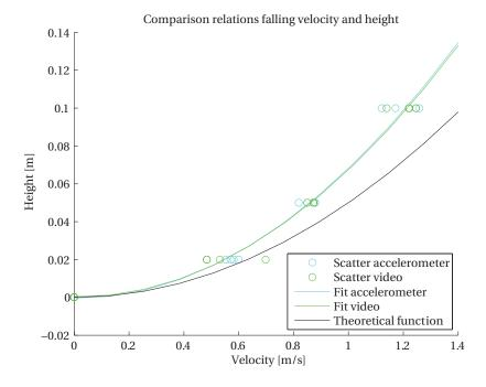
Figure E.6: Graph comparing the falling velocities from the accelerometer, camera and from theory
