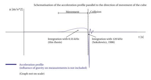
Figure 4.7: Differences in measurements of this Master's thesis in comparison with Sokolewicz (1986)
