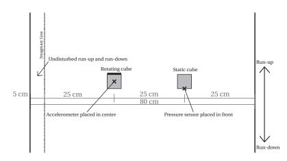
Figure 4.3: Illustration experimental set-up - top view perpendicular to slope
