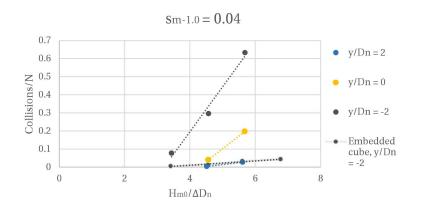
Figure 6.5: Number of collisions for steepness  $s_{m-1.0} = 0.04$
