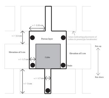
Figure 4.6: Detailed illustration of embedded cube near cube
