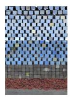
Figure 4.4: Regular placement single layer cubes (Van Gent & Luis , 2013) - top view of physical model
