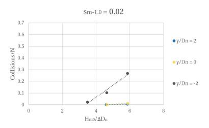
Figure 6.6: Number of collisions for steepness  $s_{m-1.0} = 0.02$
