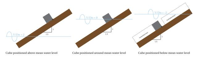
Figure 4.2: Position cube relative to mean water level - side view
