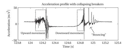
Figure 5.5: Indication upward and downward movement in accelerometer data
