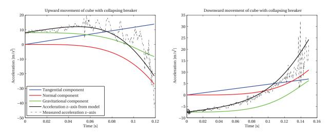
Figure 5.4: Comparison synthetic model with measured signal for collapsing breakers, extreme case
