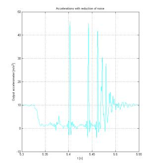
Figure E.4: Measurement of accelerations for test with falling height of 2 cm
