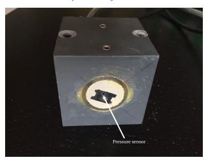
Figure C.7: Placement of pressure sensor in the center of the front face of the cube.
