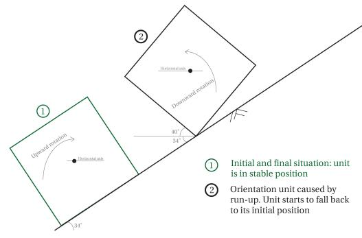
Figure 3.2: Rotations of the armour unit
