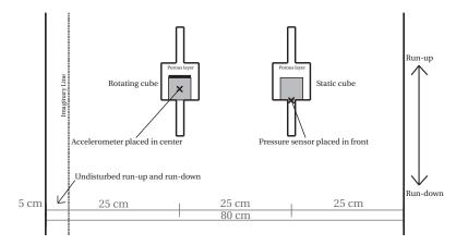
Figure 4.5: Illustration experimental set-up with embedded cube - top view perpendicular to slope
