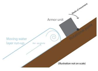
Figure 3.1: Wave run-up on slope with protruding element
