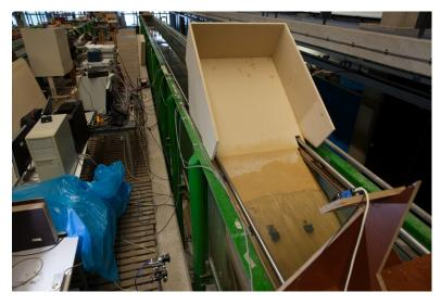
Figure C.1: Test set-up with series for exposed cubes. The slope provides undisturbed wave run-up
