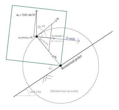
Figure 5.2: Decomposition acceleration signal for cube moving upward
