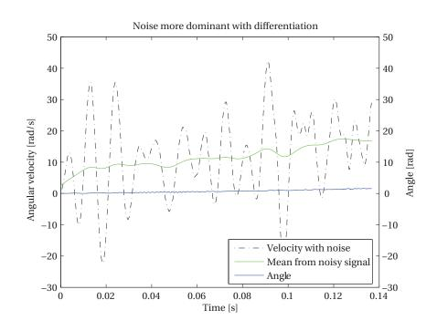
Figure 5.6: Velocity signal in time, showing the influence of noise
