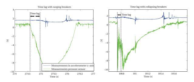
Figure 6.8: Comparison time lag between wave impact and start of movement
