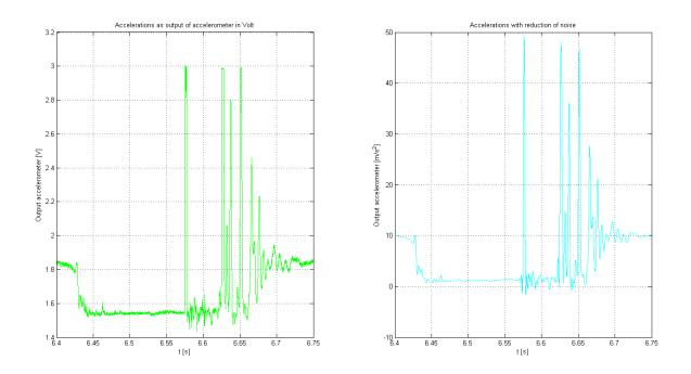
Figure E.5: Measurement of accelerations for test with falling height of 10 cm
