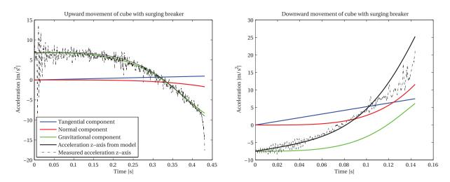
Figure 5.3: Comparison synthetic model with measured signal for surging breakers
