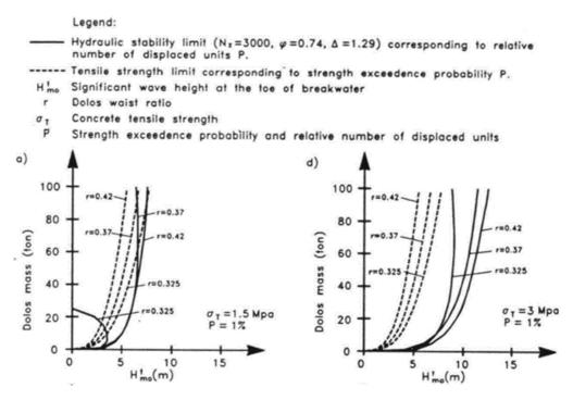
Figure 2.4: The determination of the Dolosse dimensions from design graphs (Burcharth , 1992)
