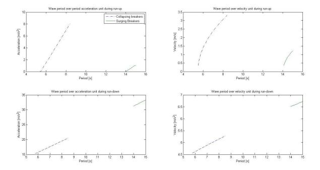
Figure I.7: Resulting accelerations and velocities varying over wave period of prototype Hexapod with orientation 1
