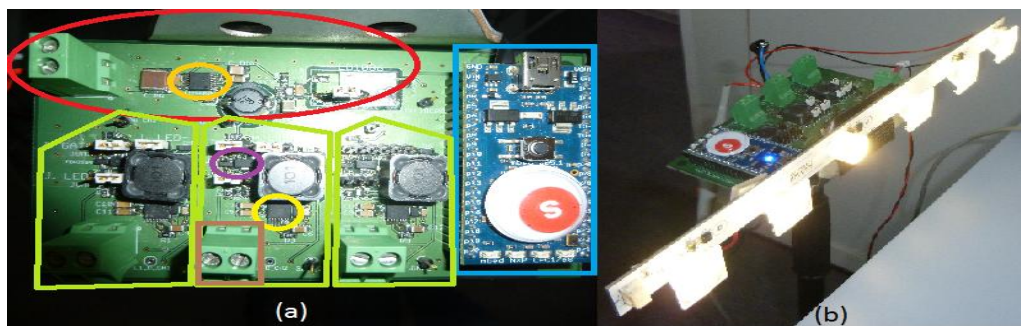
Figure 2. Picture of the transmitter: (a) Top view of the circuit made out of a 24 V supply and a dc-dc converter stage (red ellipse) with the dc-dc converter chip (orange ellipse), a microcontroller (blue rectangle) and three channels (green polygons) in which there are two different eligible MOSFETs (violet ellipse), a driver (yellow circle) and a connector (brown rectangle) for the external LEDs; and (b) a picture of the whole transmitter formed by the circuit and the external LEDs connected (in this case to channel number 2).
