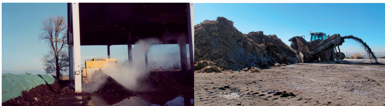
Figure 5.5.3 and 5.5.4. Windrow composting: turning machinery.
