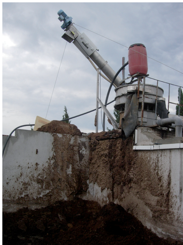
Figure 6.8.1. Separation system and composting pile of the pig farm in the tested scenario.
