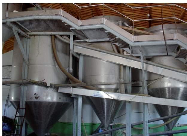
Figure 5.2.2. Cylindrical settler with conical base.
