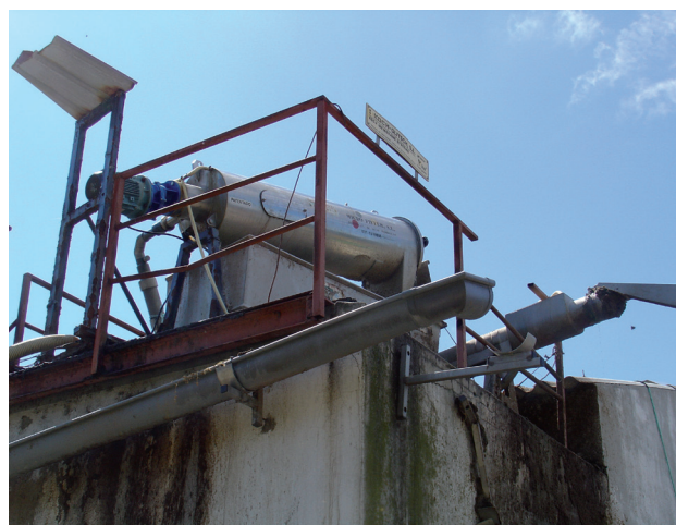
Figure 5.2.6. Screw pressing in a pig farm.
