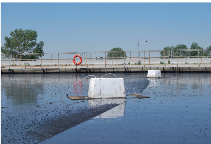
Figures 6.2.7 and 6.2.8. Emission measurements in the uncovered and covered lagoons in the treatment plant of Purines Almazan, SL (Castilla y León, Spain).
