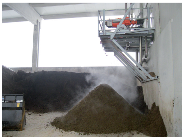
Figure 2.3.2. Phase separation (screw press). View of solid fraction.
