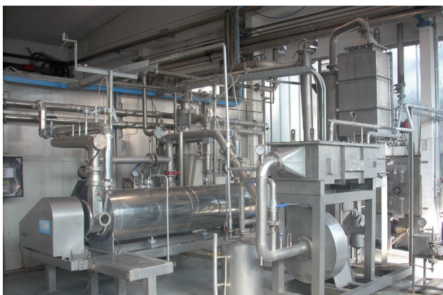
Figure 5.7.5. TurboDryer with internal high speed rotor. VOMM - Milano, Italy (CRPA, 2013).
