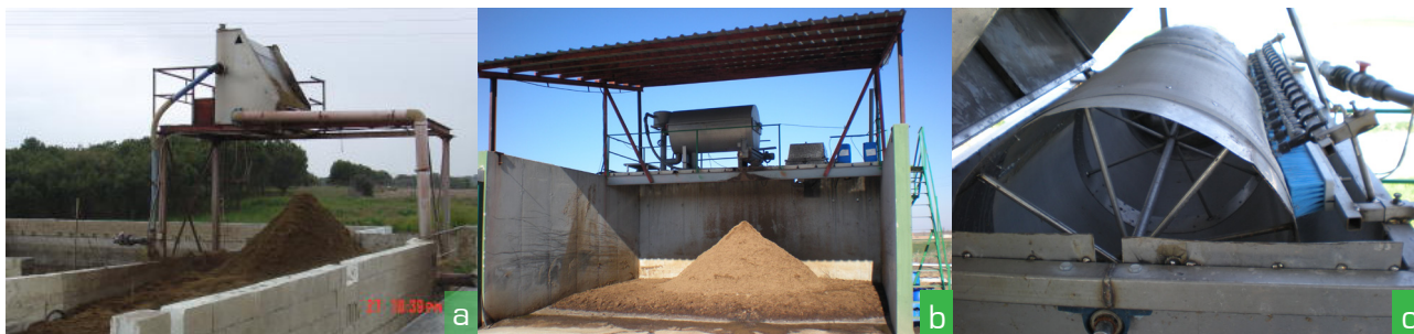
Figure 5.2.4. a) Static screen installed in a dairy farm; b) and c) rotary screens.
