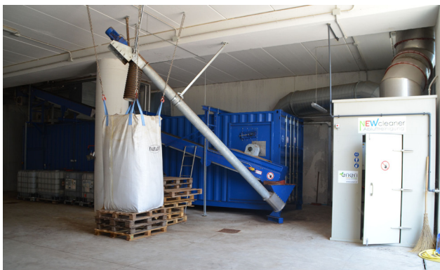
Figure 5.7.4. Dryer plant: close chamber (blu) with inside the holding belt system, scrubber box (white) and big bag filled with dried digestate in front of flubox with ammonium sulphate solution. San Giuliano farm - Trento, Italy (CRPA, 2013).
