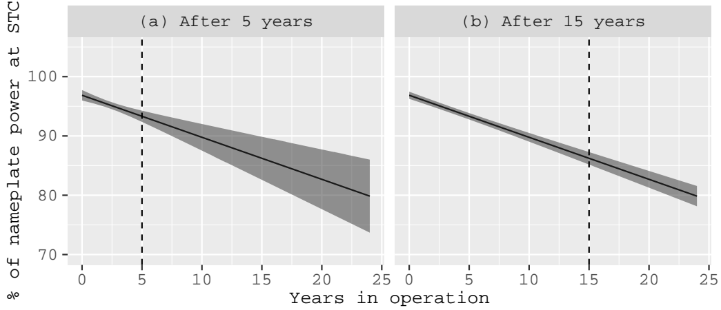
Figure 3. The 95% confidence intervals of 0.50 degradation quantile based on 5 and 15 years of data. The estimated 0.5 quantiles are shown as the solid black line. The shaded regions denote the confidence intervals.
