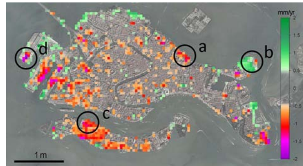
Figure 5. Quantification of man-induced ground movements obtained by removing the C-band interpolated map from the X-band interpolated solution.
