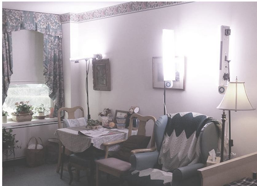
2.2 Lighting system to provide high circadian stimulation
