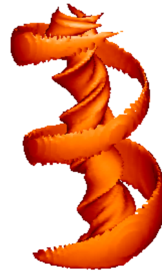
Fig. 17. An isosurface of the current for Case 2 at t = 60 showing the kinked central column of current with a helical current concentration wrapped around it.
