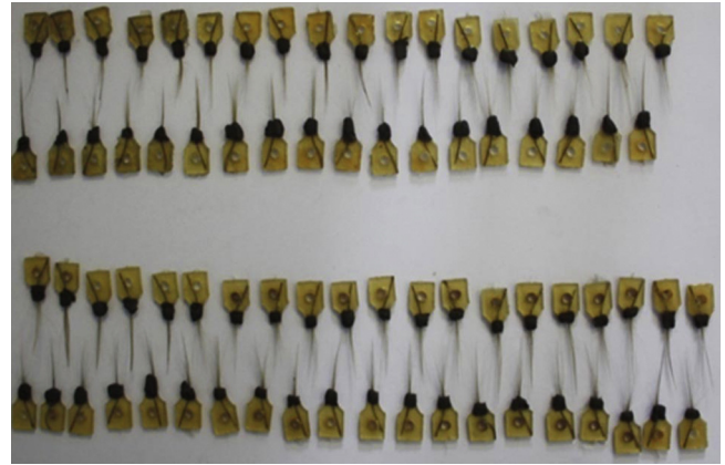
Fig. 8 – The roving after testing on long-term strength.
