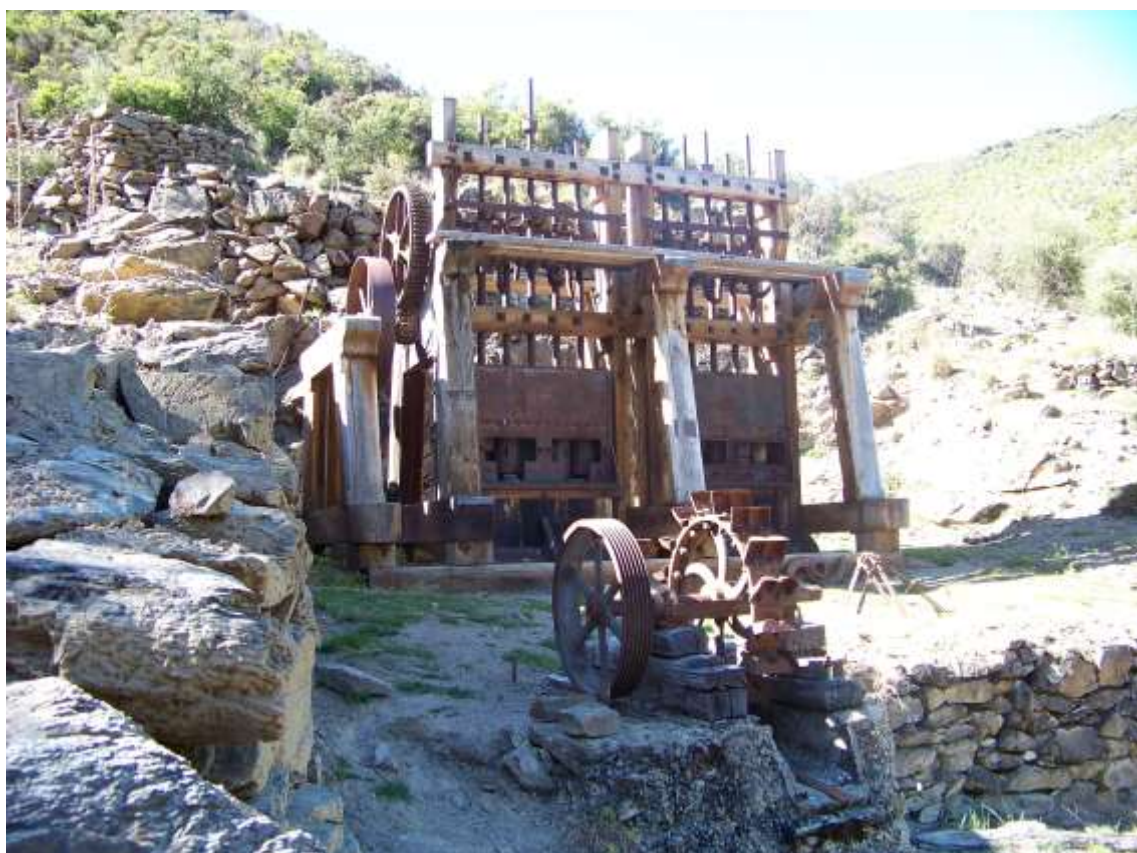
FIGURE 6a & b the old and the Repaired 1908 Come in Time Quartz Battery, L. Carpenter 2012
