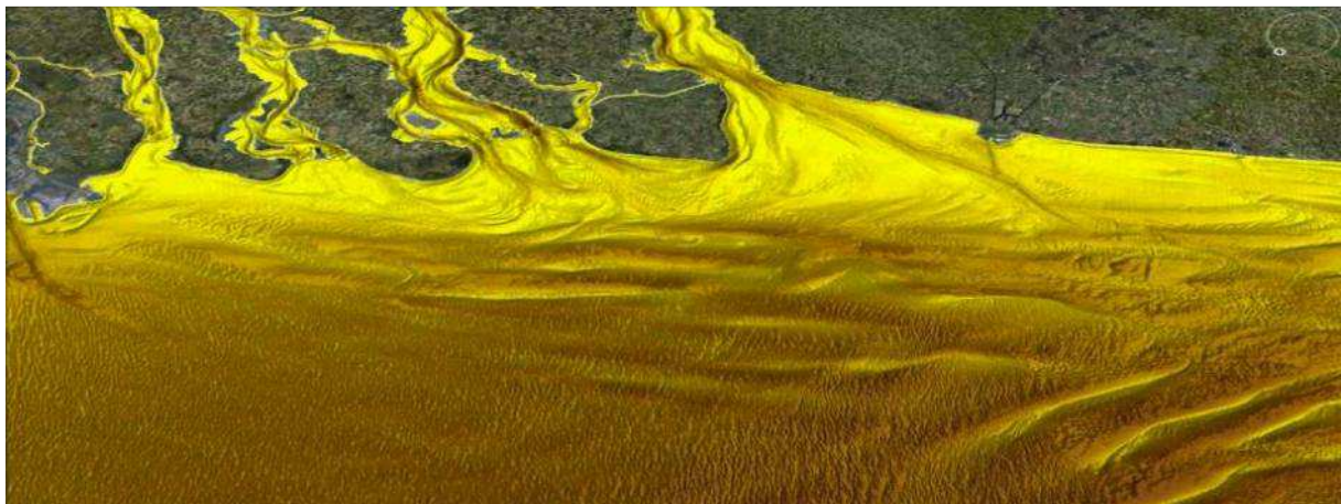
Figure 1: The Belgian-Dutch offshore area considered in the TILES project: significant volumes of sand are stored in the ebb delta of the estuaries and in sandbanks located farther seaward. North is to the West of the figure; bright to darker yellow represents shallow to deeper depths. Bathymetry data: Flanders Hydrography and Dutch Hydrographic Service & Deltares.
