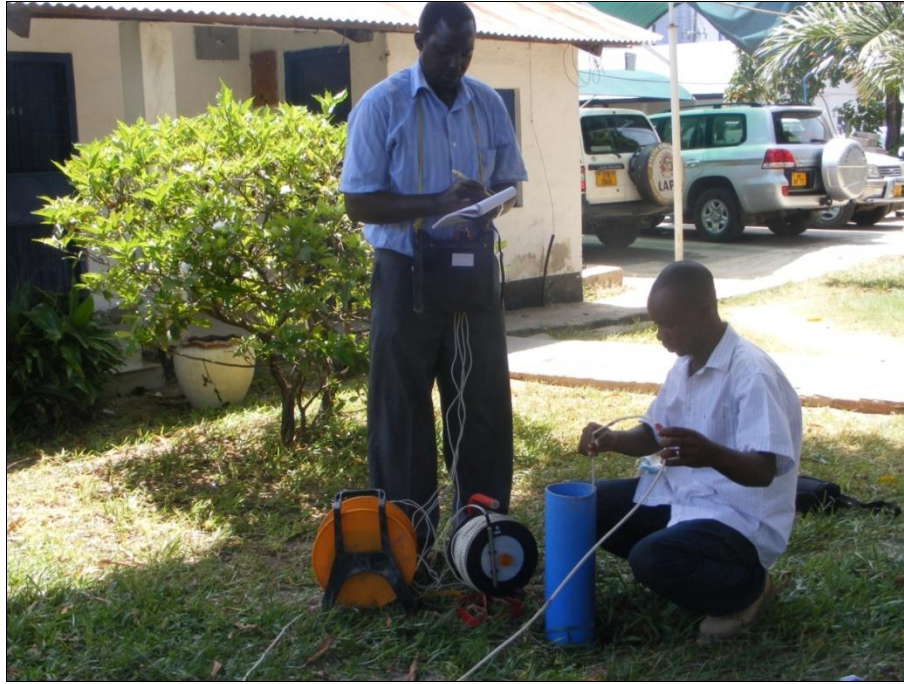
Figure 5.5: Resistivity logging (Borehole B10) at Civil Servant Service Offices, Dar es Salaam.
