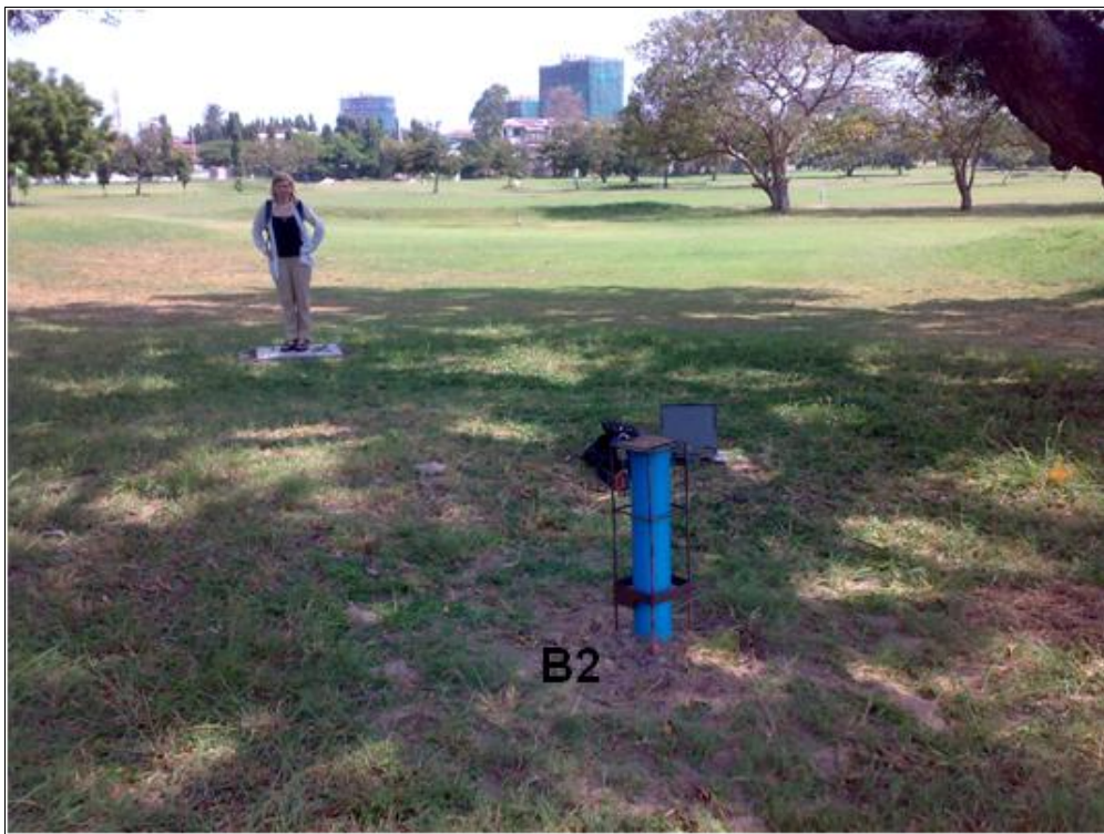
Figure 4.35: Gymkhana Golf Club production borehole covered by a concrete slab (a fellow researcher standing right on top of it) and monitoring borehole B2 (installed with Mini-Diver (50m) J02701).
