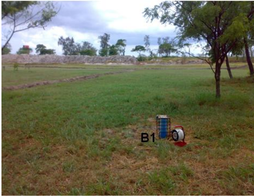
Figure 4.31: Borehole B1 located at about 0.22 km from the ocean, since 27 February 2011 was equipped with Mini-Diver H0461 for monitoring water level and temperature. The Mini-Diver was replaced by CTD-Diver K6627) on the 7 July 2011.
