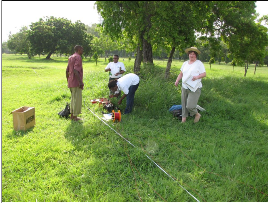
Figure 5.3: Setting ABEM Terrameter SAS 1000 before starting measurements at Gymkhana Golf Club (January 2012).
