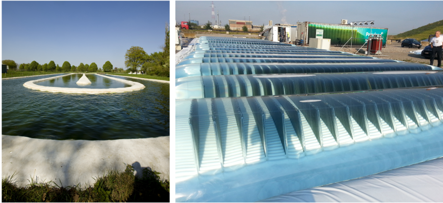
Figure 1.3: Example of open raceway pond reactors (Ingrepro, The Netherlands) and a novel design of a low-cost photobioreactor (Proviron, Belgium) [187].
