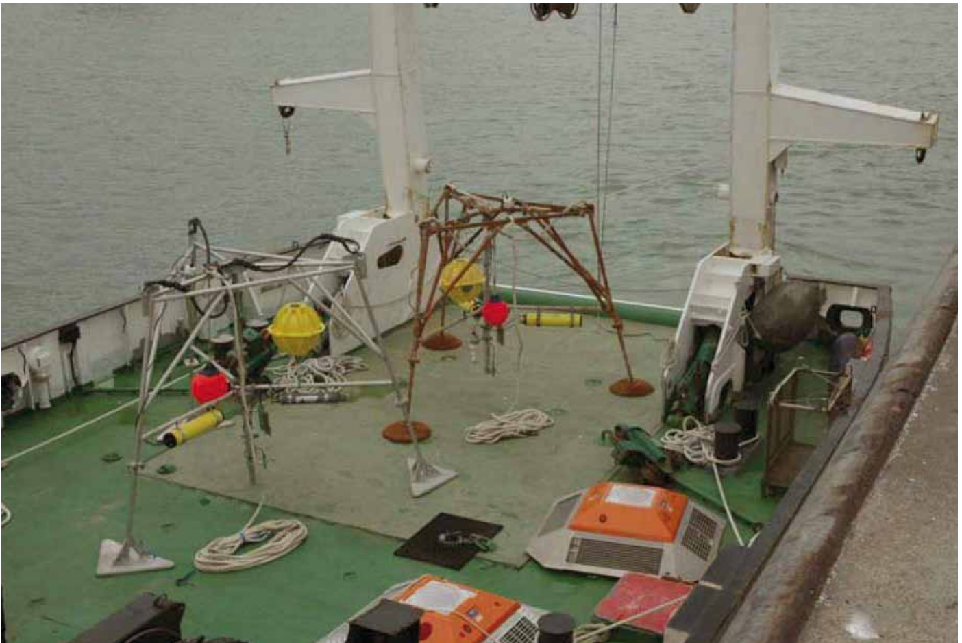
Figure 3. Two tripods and two ADCPs ready for deployment on the Bligh Bank and the Gootebank (RV Belgica).
