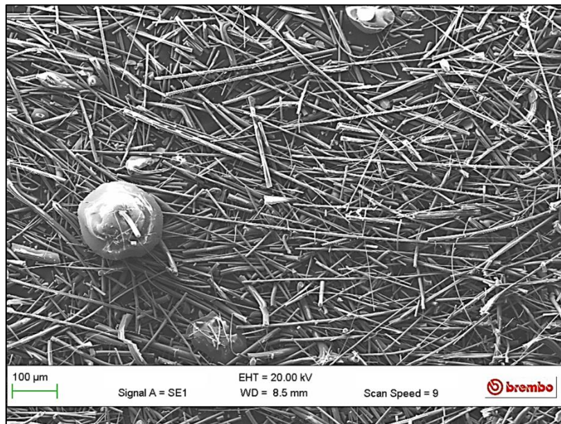
Fig.2.57 SEM image of a Man Made Mineral Fiber, big spherical shots can be easily distinguished from fibrous elements.
