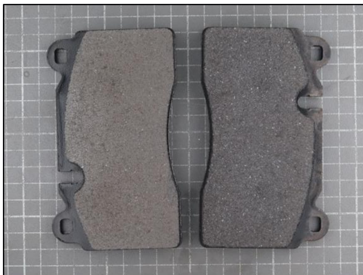
Fig.3.12 Organic (on the left) and inorganic (on the right) brake pad
