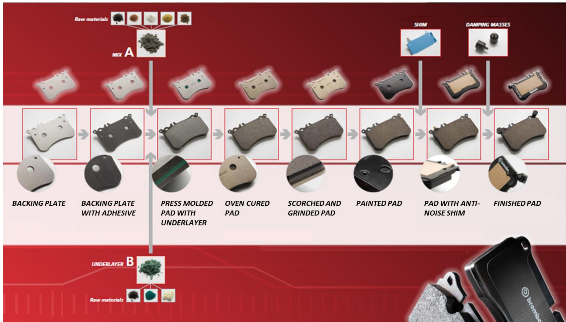
Fig.3.7 Main manufacturing steps of commercial organic brake pads. (Courtesy of Brembo S.p.A.)
