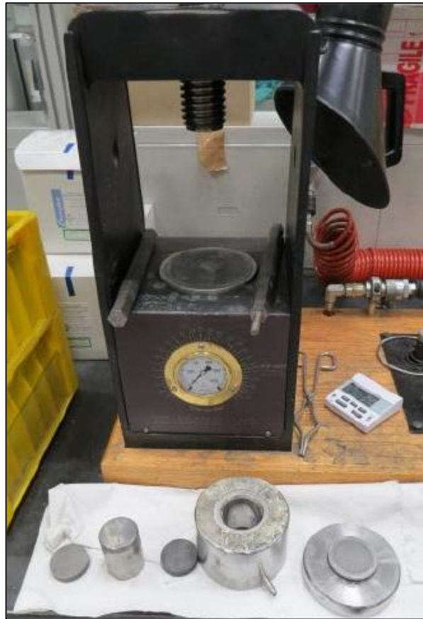
Fig.3.9 : Pressing machine E-Z™ 40 used for laboratory scale samples preparation
