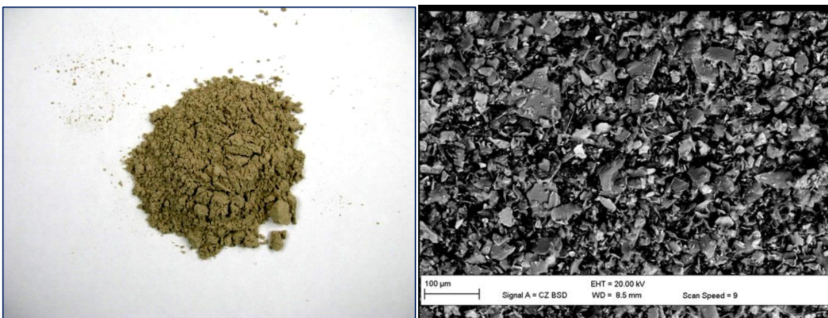
Fig.3.3 Phlogopite mica, powder aspect on the left and SEM-BSD images on the right
